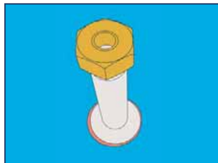
4 Wipe excess sealant from around flange.
