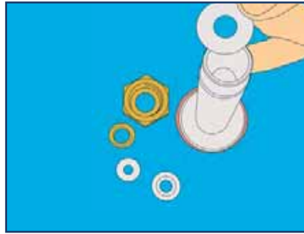
7 Size washers to cable & insert if required.
