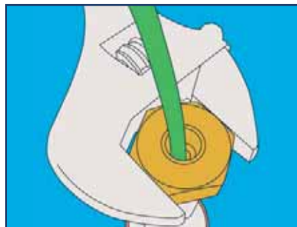
12 Push cable through assembled gland & tighten nut.
