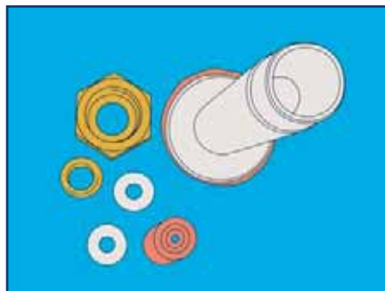
5 Remove top nut & internal parts.
