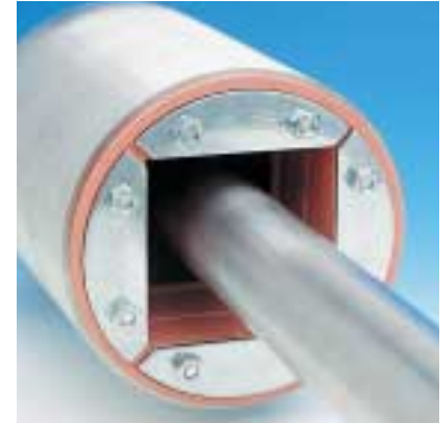
1. The RGP plug is mounted in the sleeve, which is welded or bolted to the deck or bulkhead. The pipe is then pulled through the RGP plug. Open RGPO plugs are used if the pipes are already in place.
