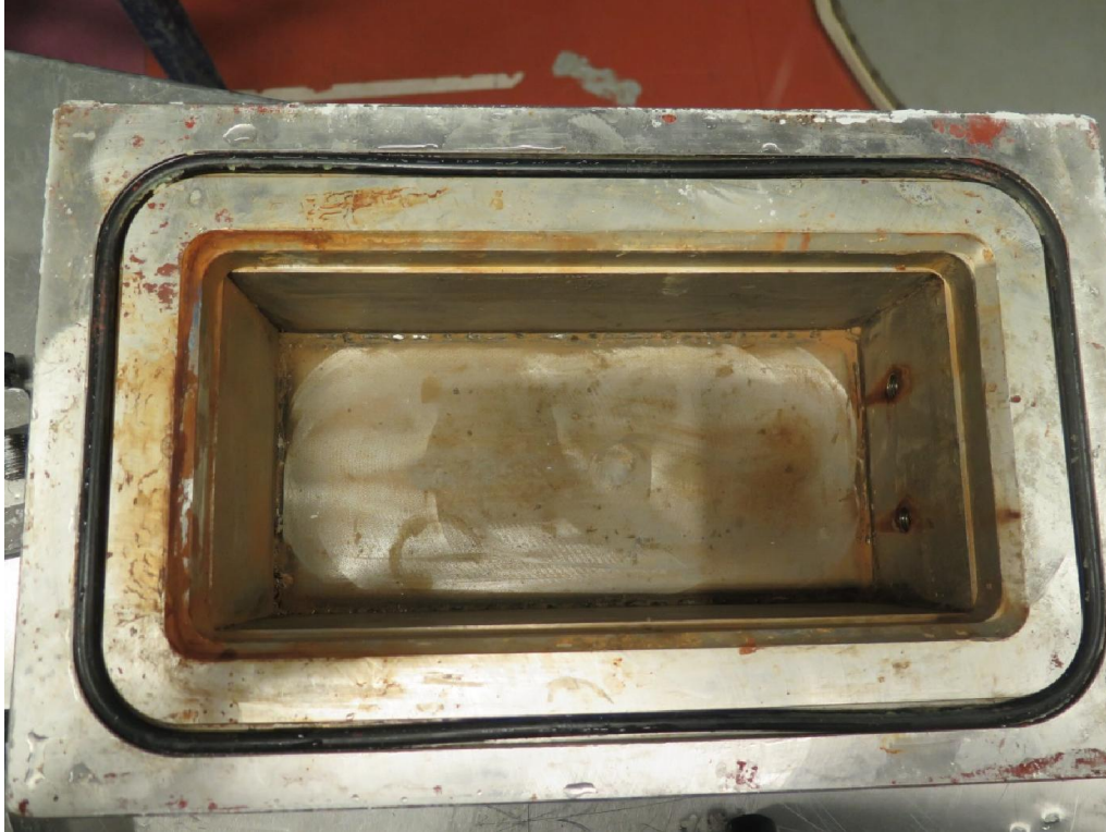
Picture 10: No trace of water inside the EUT after the IPX5 test
