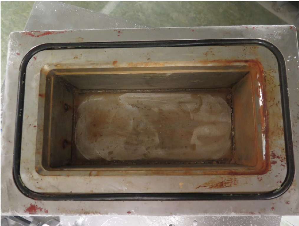
Picture 7: No trace of dust after the IP6X test
