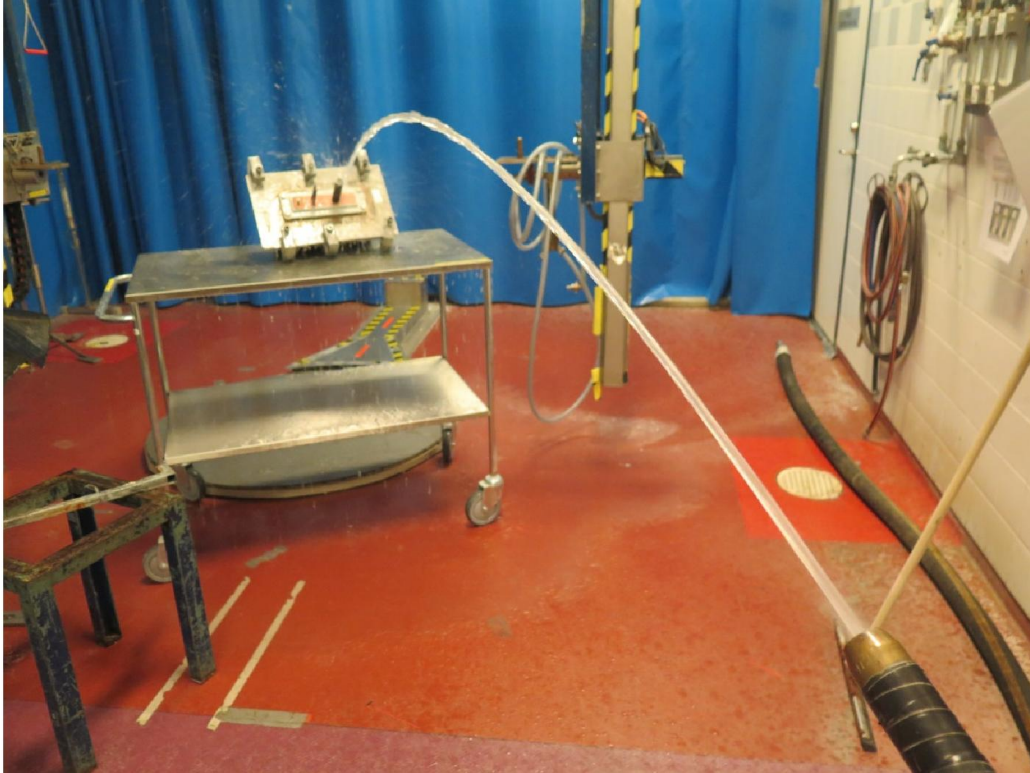
Picture 8: EUT during water jet test (IPX5)
