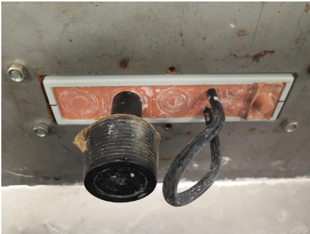
Picture 9: No trace of water inside the EUT after the IPX5 test
