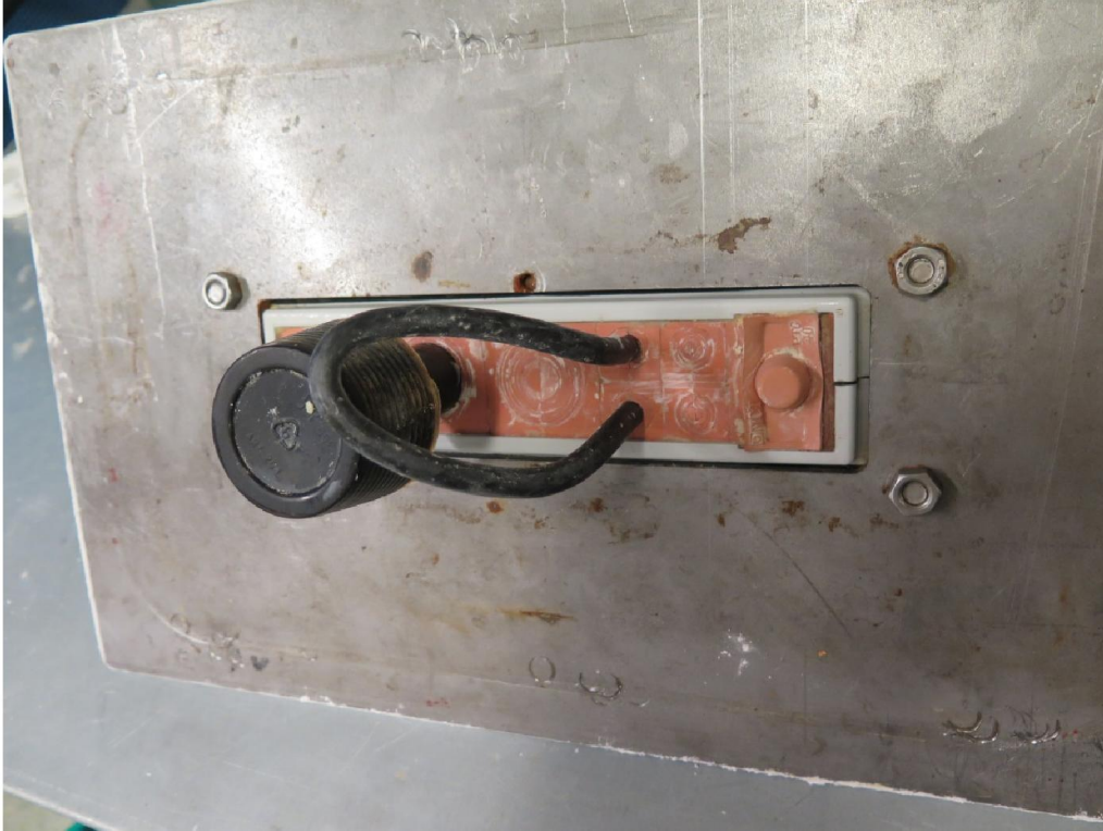
Picture 6: No trace of dust after the IP6X test
