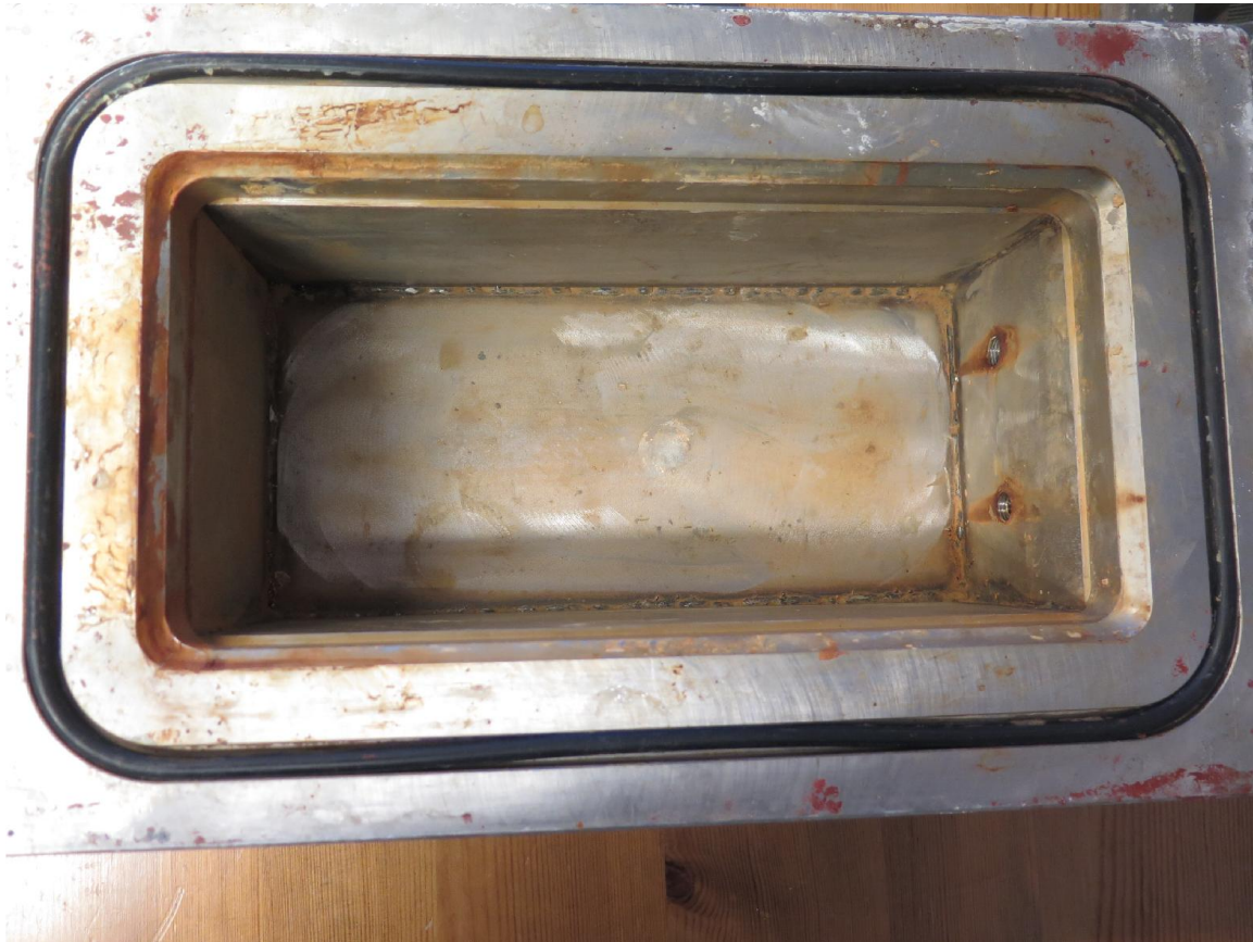
Picture 13: No trace of water inside the EUT after the IPX7 test
