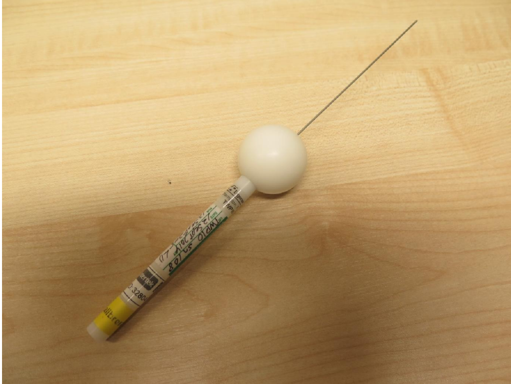
Picture 2: Test probe \varnothing 1.0 mm for IP6X-test
