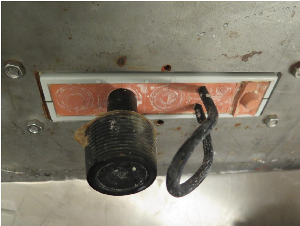
Picture 12: No trace of water inside the EUT after the IPX7 test
