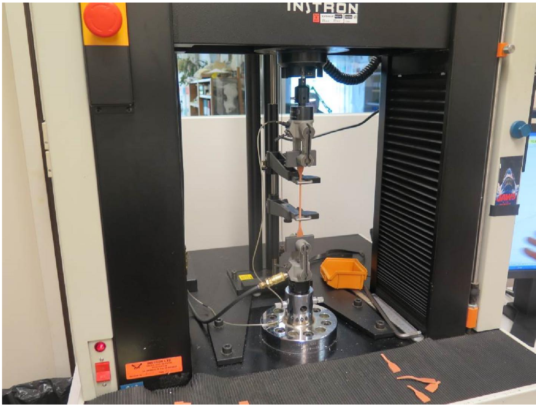
Picture 5: EUT during tensile strength and elongation tests
