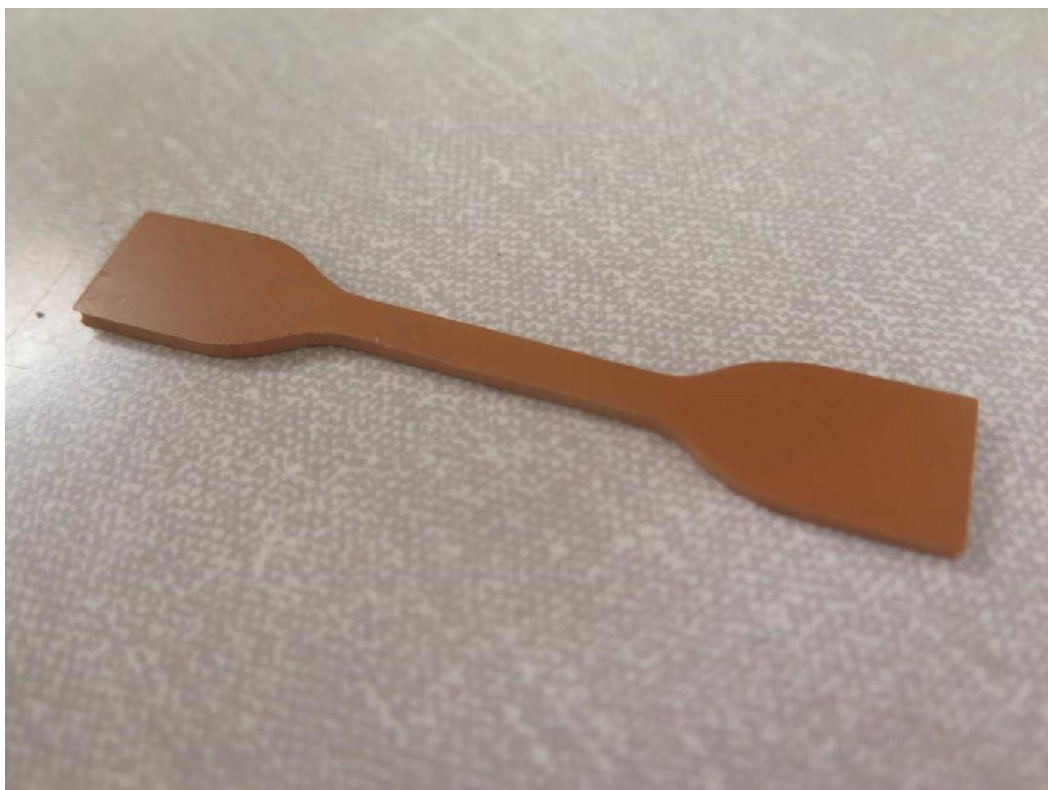
Picture 4: Dog bone used for tensile strength and elongation tests
