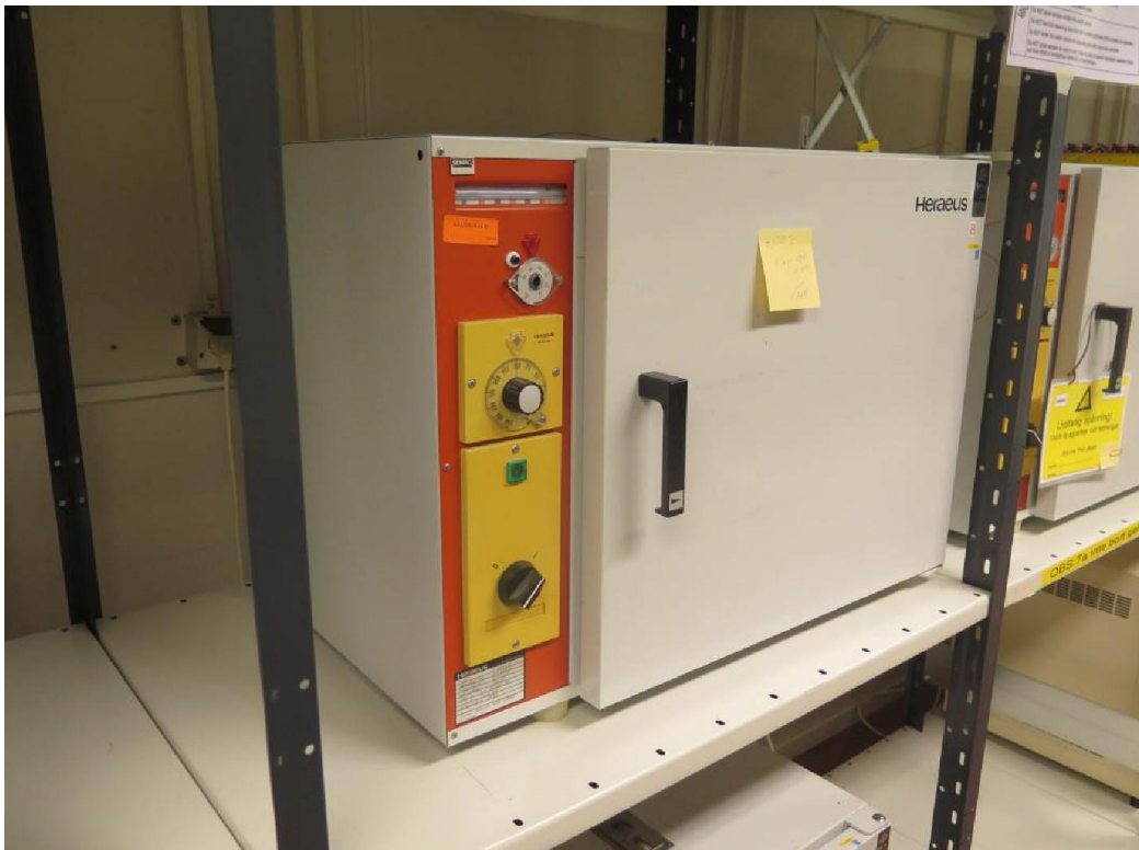
Picture 3: Temp chamber used for 70°C circulating air for 168 hours
