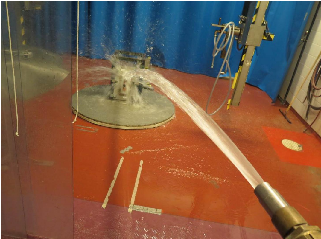
Picture 2: EUT during water hosedown test
